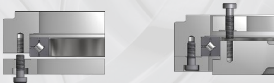
Mounting Crossed roller bearing with clamping rings
